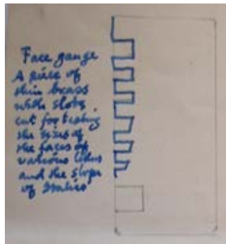
Fig App. K.1: Face gauge as described by Harry Carter (St. Bride Library)
