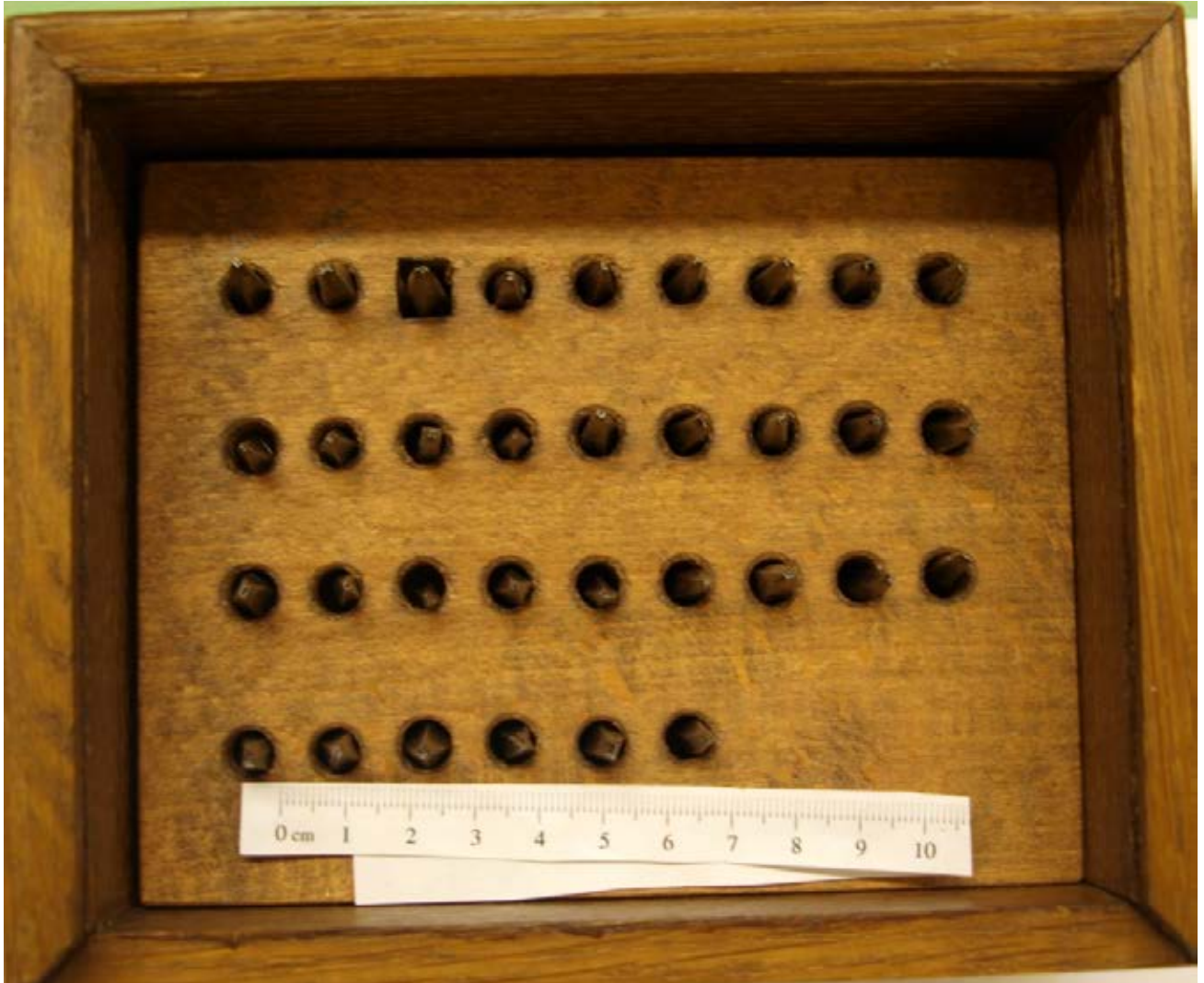
Fig. 3.53: Hb 15 (S): Complete set of punches for ST 55 showing the image end. Slightly reduced in size (Museum Plantin-Moretus/Prentenkabinet)
