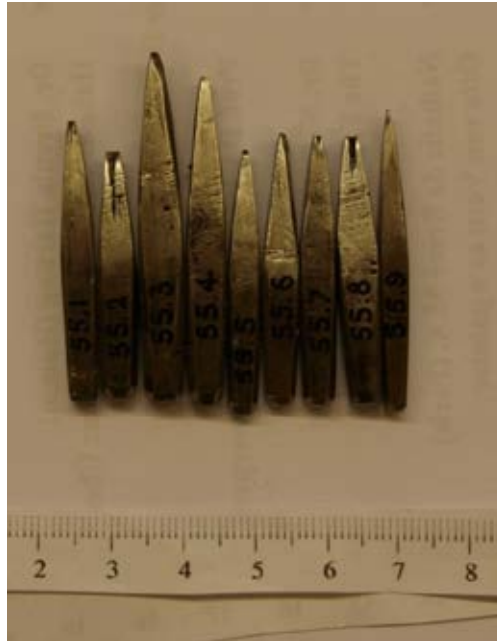
Fig. 3.54: Hb 15 (S): Selected punches from ST 55 showing differing punch heights and finish. (Museum Plantin-Moretus/Prentenkabinet)
