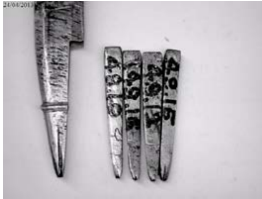
Fig. 2.38: ST49 Jolie Grecque Granjon showing lower case character stepped punch with four accents
