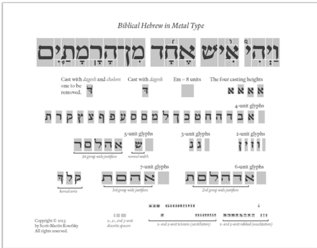
Fig. 4.30: Biblical Hebrew setting schema for metal type. (By permission of Scott-Martin Kosofsky)
