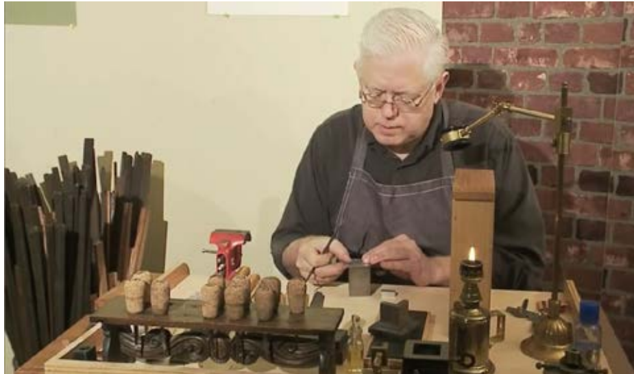
Fig. 1.2: Inscribing the character on the head of the punch – A clip from Stan Nelson video Punchcutting at the Atelier Press & Letterfoundry
