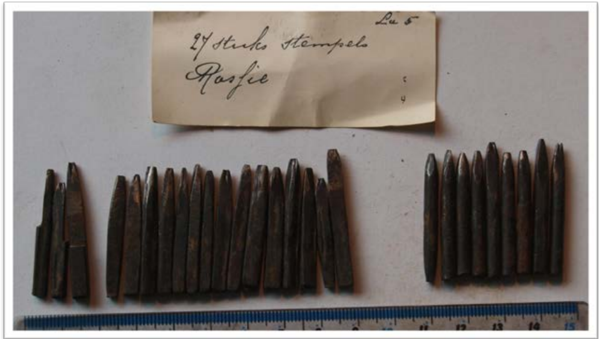
Fig. 2.35: Stepped and normal Rashi Script punches from the Athias Cabinet (Drawer 5). (The University of Amsterdam Special Collections)
