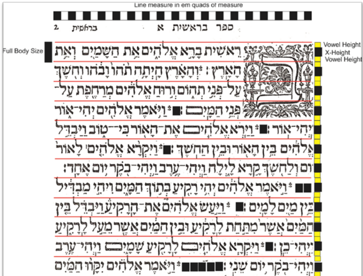
Fig. 3.39: Hb13 (S) Diagram of Body size, x-height and line spacing from the Plantin Polyglot Bible. Actual size (BL 6.h.4-11.)
