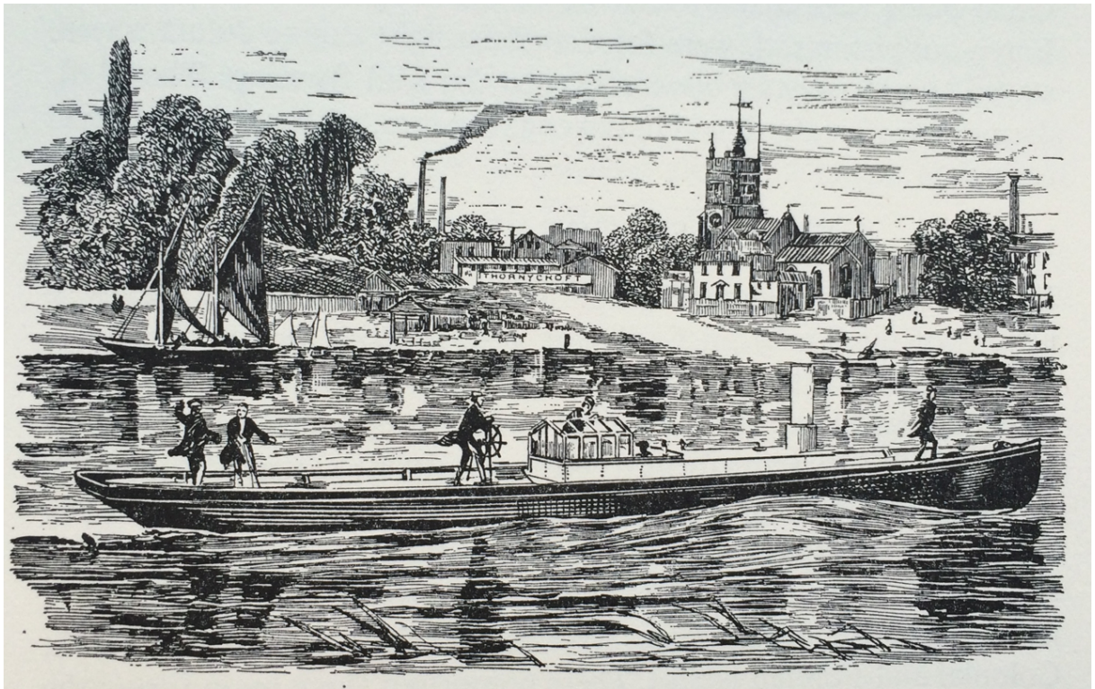
Figure 17: Speed testing 'The Sir Arthur Cotton' in Chiswick (1874). The London Journal said she was the fastest vessel in the world with a trial speed of 21.4 knots. 5
