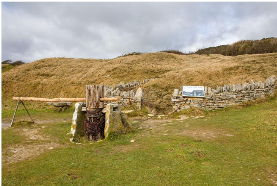
Figure 20. Old winch at a quarry in Durlston, Dorset, with a vertical axis. This would have been powered by a horse or donkey.
