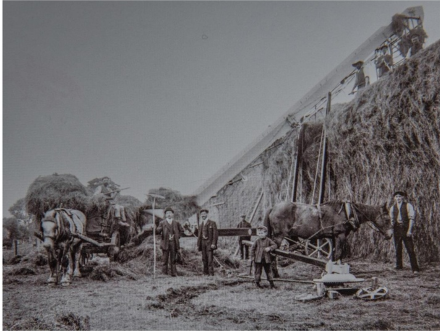
Figure 89. Mechanised farming 1907 – use of horse-driven gin/motor to drive a conveyor belt to build haystacks.
